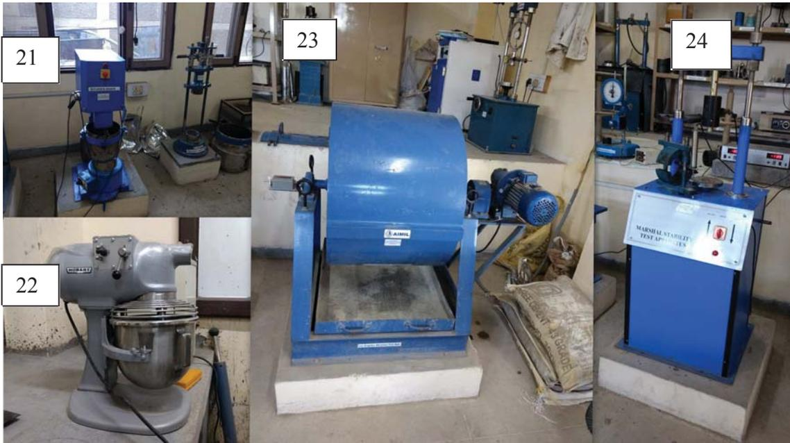
21. Bitumen Mixer/ Impact Testing Machine
