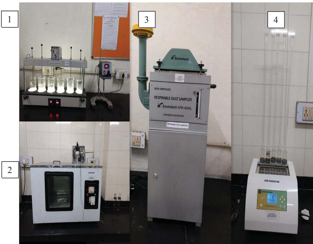
1. Jar Test Apparatus      2. Hot Bath Apparatus      3. Respirable Dust Sampler
