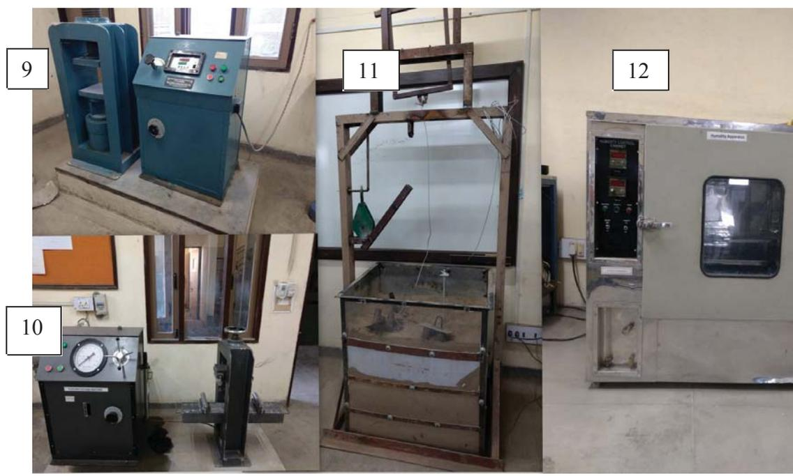
9. Compression Testing Machine 10. Flexural Strength Testing Apparatus
