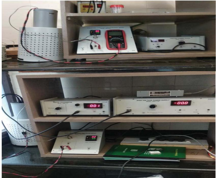
Two Probe Experimental Setup for Resistivity Measurement at different temperatures.
