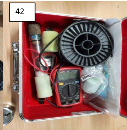
42. Half cell potential tester
