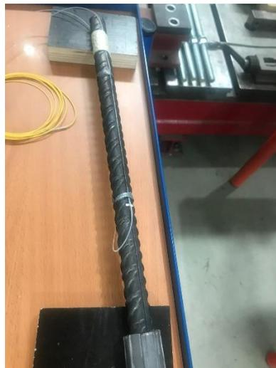
**Photo:** Observing Behaviour of Reinforcement Bar using Optic Fibers
