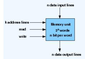
**Internal Construction:** The internal construction of a random-access memory of m words with n bits per word consists of m\*n binary storage cells and associated decoding circuits for selecting individual words. The binary cell is the basic building block of a memory unit.
