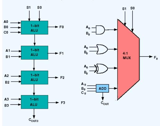
The 4-bit ALU block is combined using 4 1-bit ALU block
